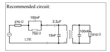
In practice, the  $910\Omega$  load resistor will connect to a low output impedance TX driver. The 100nF capacitor should appear in parallel with the  $910\Omega$  load resistor (rather than in parallel with transformer winding) toobtain optimum TX flatness to line.
